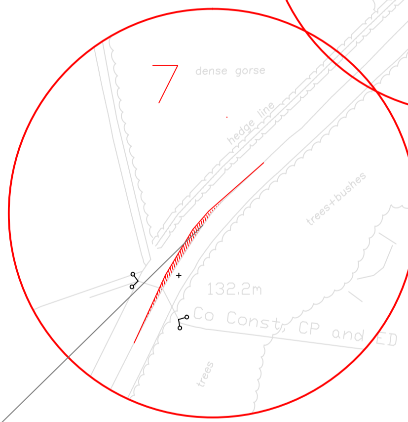
Existing tarmacadam carriageway width 4.3m. Widen damaged verge 1.2m max widening over 60m length to follow existing highway curve
